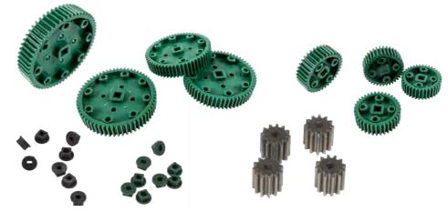
This kit features gears designed to handle higher loads. Each of these gears has a wider face width; this means each tooth is wider so applied loads will be spread over a larger area.
