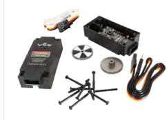
Designed to provide you with direct and detailed information from your robot's motors, the Integrated Encoder Module installs easily by replacing the plastic cap on your 2-Wire Motor 393. You can then use programming software to read what direction your motor is moving, how fast, and number of rotations.
