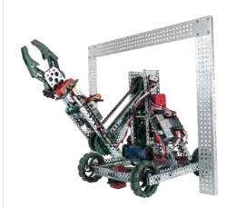
Designed to quickly determine if a VEX Robotics Competition Robot fits into the 18" maximum sizing dimension. This sizing bracket does not require the robot to be sitting on a baseplate, and can be used to measure a robot on any surface.
