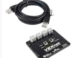
Enable/disable up to four VEXnet robots This switch also has the ability to toggle between autonomous & operator control mode. Use this kit to simulate a VEX EDR field controller for match practice!
