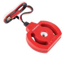
Can determine both the absolute position and direction of rotation. This measurement can help to understand the position of robot arms or other mechanisms using programming software. Potentiometers are typically used for "limited rotation" applications, such as an arm or lever.
