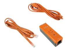
Provides a connection between your PC and a VEX ARM® Cortex®-based Microcontroller. When used with the VEX ARM® Cortex®-based Microcontroller, the programming cable allows you to monitor sensor values, perform live debugging of the code, and execute wireless downloads between the microcontroller & PC.
