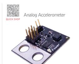
Measures accelerations on three axes simultaneously. By measuring the acceleration of the robot, one can calculate the velocity of the robot or the distance the robot has traveled. Accelerometers are also great for detecting collisions and determining if the robot is stopped or moving.
