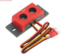
Avoid obstacles and measure distances with the ultrasonic range finder. This device emits a high-frequency sound wave that alerts the robot to obstacles in its path.
