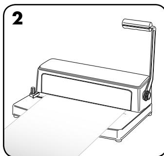
Test punch scrap sheets to check edge guide setting.
