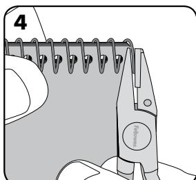
Use the binding pliers to cut the end of the metal coil. Clip off the excess coil.
