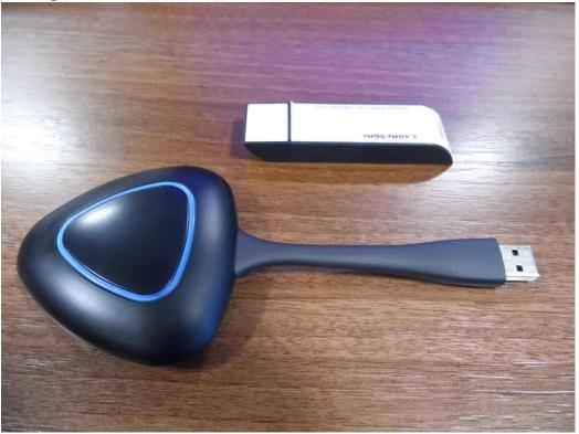
For clarity the top unit is the receiver and the lower unit is the transmitter.
