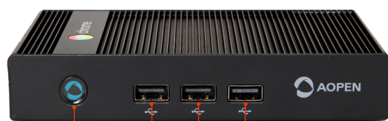
Power Button USB 2.0 w /BC1.2, each port supports 5V/1.5A
